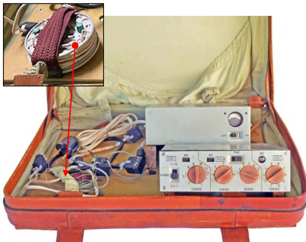
General view of the unknown Polish suitcase with the transmitter and AC mains power supply unit in position. It is believed that a high speed keyer and possibly a receiver was part of a station.
