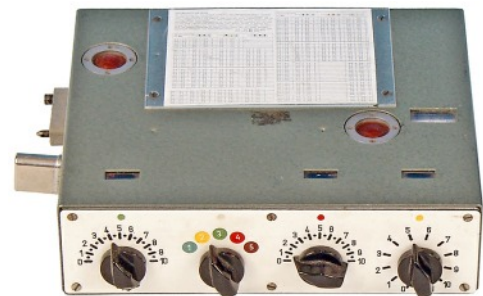
The SE 25, also known as 'Elbe' was an East German agents transmitter. It was used in combination with a NE 25 AC mains power unit or a 12V DC transverter, and a high speed Morse Keyer 'Geber E' (See Chapter 60).
